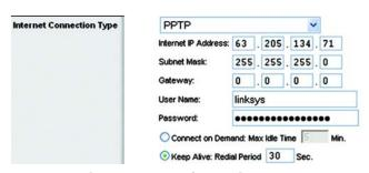
**Figure 8-6: PPTP Connection Type**
